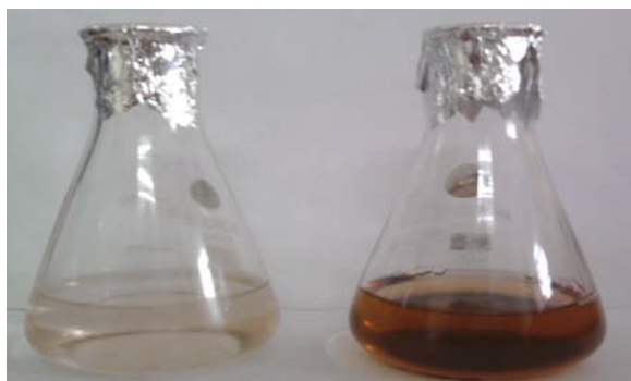
Fig. 2. Picture of aqueous solution of 1mM \text{AgNO}_3 with Ocimum leaf extracts before adding the leaf extract and after addition of leaf broth.
